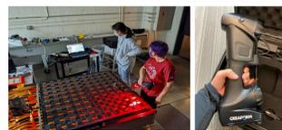
A 3D model of the RICH created by 3D scanning ▲ Scanning of the SiPMs on the focal plane ◀ the 3D scanner ▶
